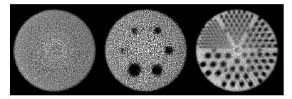
Conversely, below are "abnormal" transverse slices from a Jaszczak Phantom.
