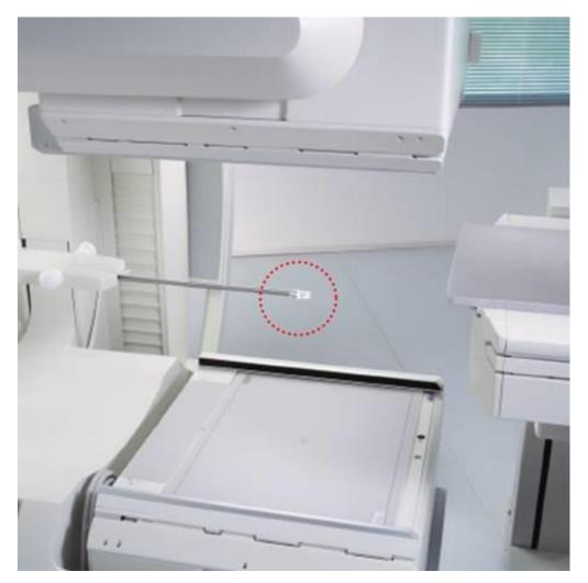
With the collimator removed, a point source "floods" a detector with radiation as shown below. This process is analogous to a flashlight "flooding" light on an object. In both cases, the closer the source to the object, the less uniform the distribution. However, the greater the distance from the source to the object, the weaker the radiation or illumination.
