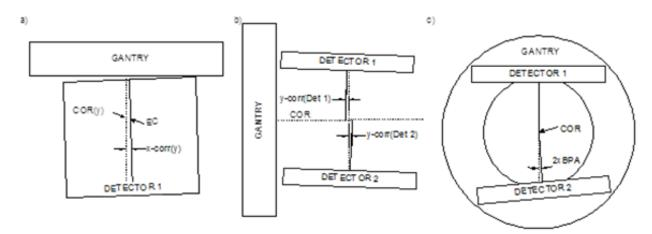
Originally, Siemens called the procedure to acquire these corrections on Dual Head cameras a Multi Head Registration. Nowadays, it's commonly known as a Head Alignment Calibration.
