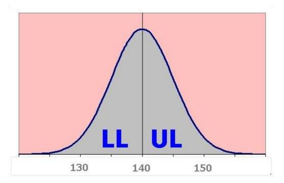
When a predetermined number of counts have been acquired in either the LL or UL within each PMT's Tune Mask, the system momentarily stops acquiring and analyzes the data. That's called a Tune Pass. The counts in each PMT's LL and UL are compared, and the result is the PMT's Tune Value.
