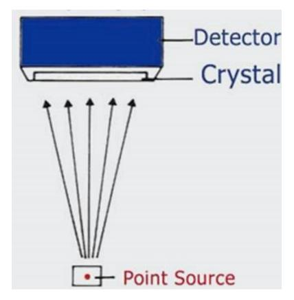
For Siemens Dual Head cameras, a technetium point source of 30 to 35 microcuries is needed and the source should be midway between the two detectors when the heads are fully retracted. For systems with AQC (Automated Quality Control) a 50 microcurie cobalt point source in initially installed in the Front Bed and then replaced on an annual basis.
