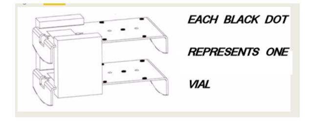
Afterwards, a SPECT/CT acquisition is preformed, and the resultant corrections align the 10 technetium points in the nuclear scan with the 10 contrast points in the CT exam. NM/CT FOC Calibrations are stored on the acquisition workstation (rather than in the SNAC or in the detector) in the GDS.mdb and BINARY DATA folder.
