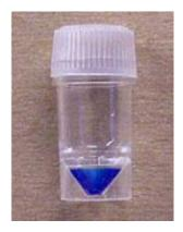
To be precise, each vial should only contain 0.15 mL or less of solution in a 4 to 1 water to contrast ratio. No cotton or other material should be placed in the vial.
